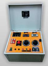
This is a Portable Testing Kit in One Unit, Suitable for Testing Protective Relay, Over Current Relay, Earth Fault Relay, Circuit Breaker, Tripping Coils etc. The set is Designed for Both Laboratory and field use.
