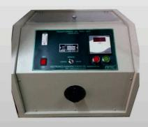
Oil test set is an equipment designed to test the dielectric strength of insulating oils as per relevant specification viz. IS 6972 it is a useful equipment for transformer/switchgear manufacturing units. Oil filtering agencies, repair shop and electrical maintenance departments.
