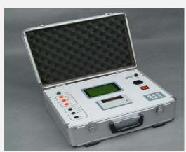
DY-100 Automatic Transformer Turns Ratio Tester is a new, fully automatic tester that measures transformation ratio of single phase and three phase transformers using modern electronic techniques and does not require any manual 'null' balancing.
